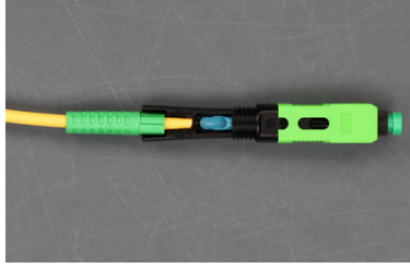
Step 12: Push the soft tail into the end of the connector. Ensure the rectangular wing is oriented upward.
