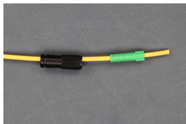
Step 1: Put boot and soft tail on cable.
