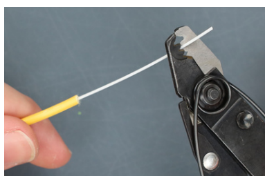
Step 5: Strip the 900 µm tubing at interface of cable. Do this in small sections at a time to avoid breaking the fiber. **Note: If the 900 µm tubing is tight-buffer, you will be left with bare fiber and will skip Step 6 and Step 7. Move ahead to Step 8.
